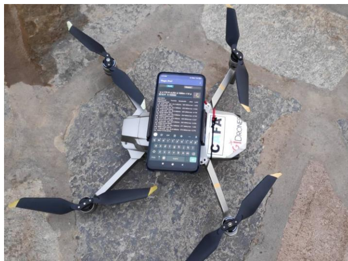
Figure 3 – 5G smartphone Xiaomi attached on CAFA Tech drone Mavic
