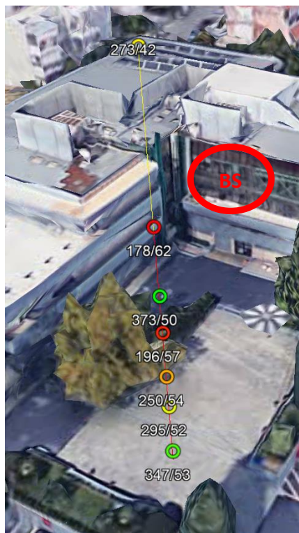
Figure 5 – OTE Acedemy-Speedtest with nPerf at levels 0-5-8-12-15-20-30 meter
